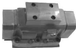
Main Shift Valve, Mechanical Shift
